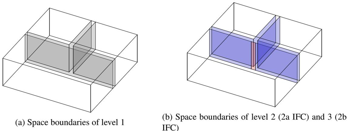
Figure 2: Space boundaries of different levels according to LBNL methodology (Bazjanac 2010) respectively IFC. Level 1 in gray, level two (2a IFC) in blue, level three (2b IFC) in red
