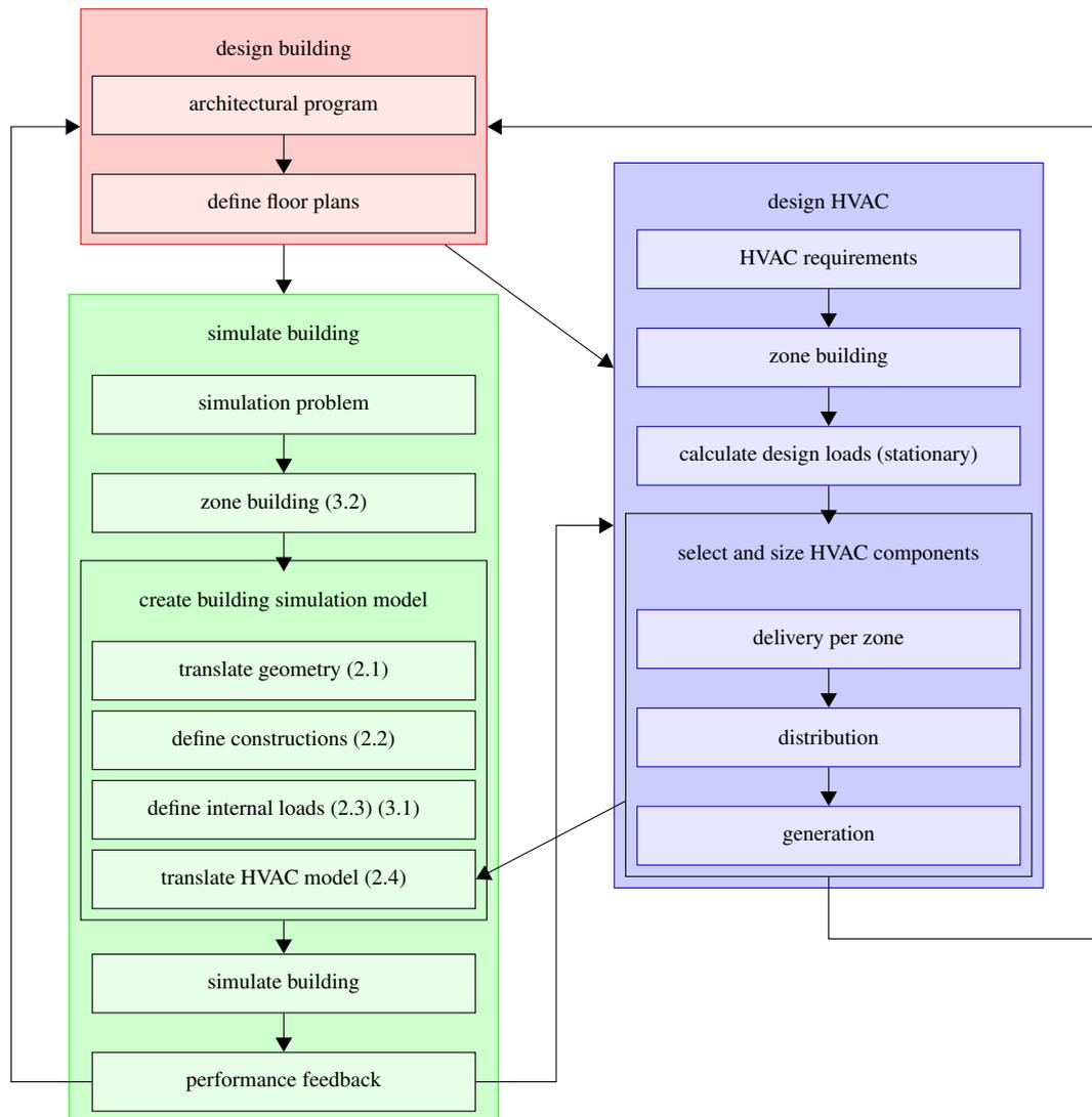
Figure 1: Workflow model for building energy simulation in the design process, with the following roles: architect (red), HVAC designer (blue), simulation user (green)
