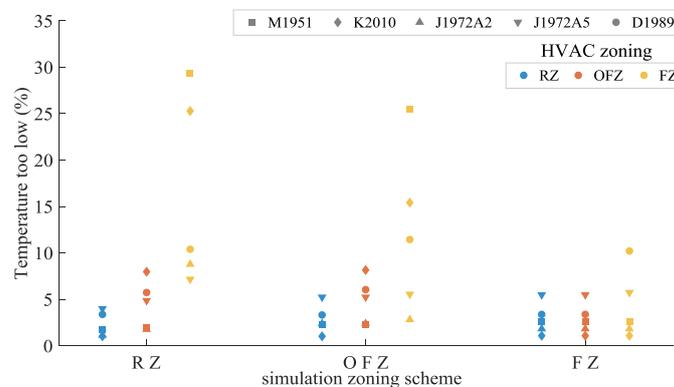
Figure 4: Proportion of time (during the simulation period January) and floor area in which simulated temperatures are lower than set point. Colors stand for HVAC zoning schemes.
