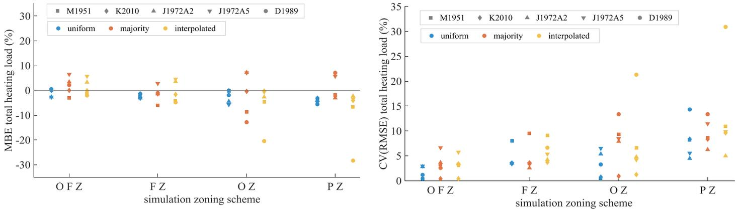
Figure 3: Error in total building heating load for buildings floors, zoning schemes and internal load variations relative to room-based zoning (RZ). Marker shapes represent building floors, and colors stand for internal load variations, as described in Table 4.
