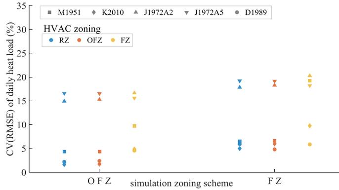
Figure 5: Errors in total heating load with several simulation zonings and HVAC zonings relative to room simulation zoning (RZ). Colors stand for HVAC zoning schemes.
