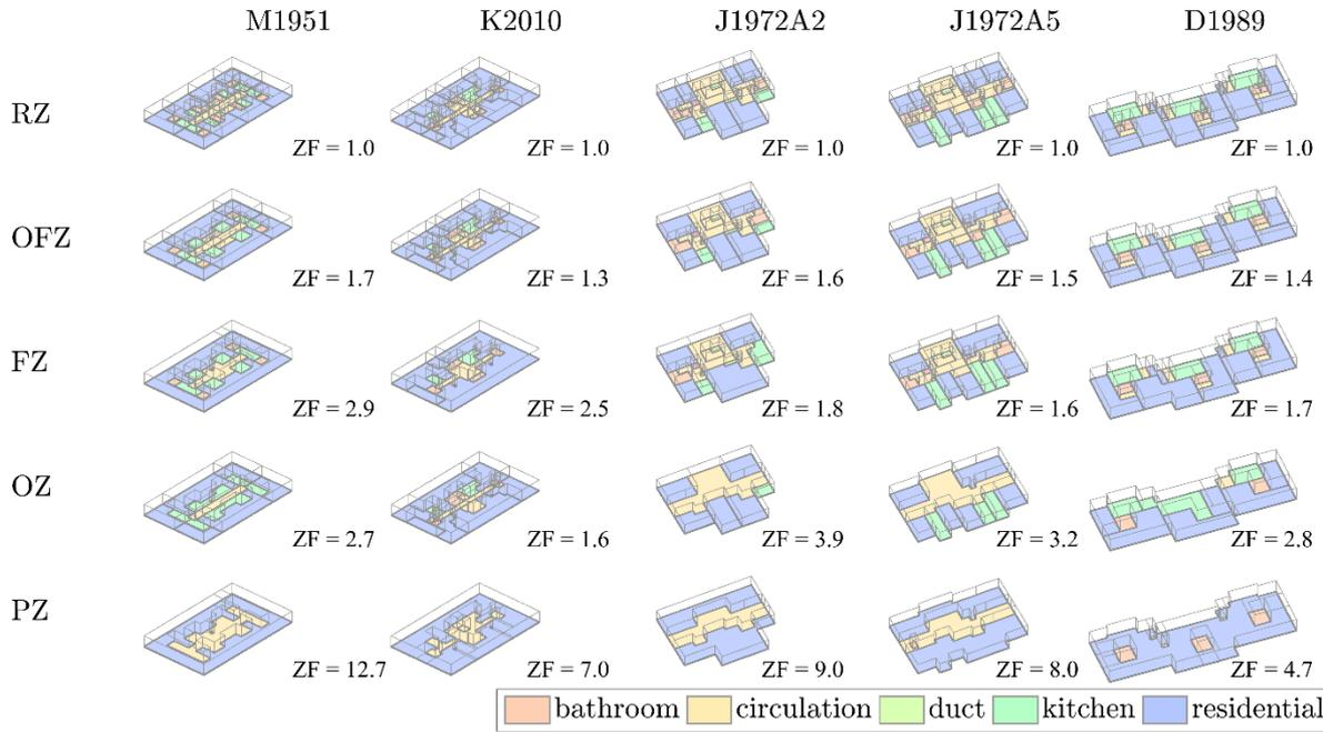
Figure 2: Resulting layouts for the selected floor models and zoning schemes, with the corresponding zoning factors (ZF).
