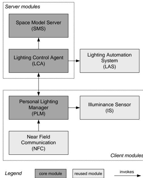
Figure 1: System architecture of the personalized, space model based lighting control system.
