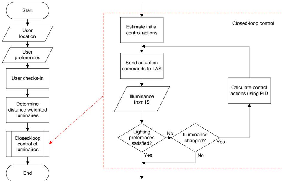
Figure 3: Single-user lighting control algorithm.
